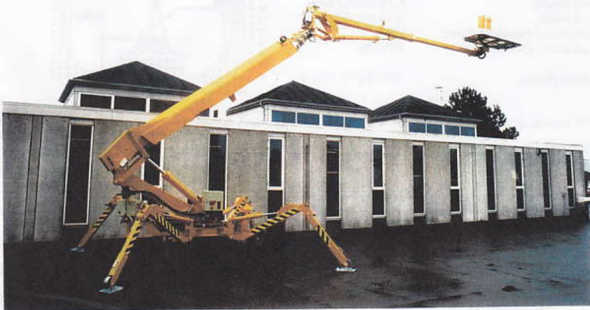
Photo: Spider TST 29, 29 m working height. Introducing new 260° articulated, telescopic jib (6 m.)
